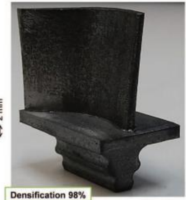
b) Spark plasma sintered turbine blade
